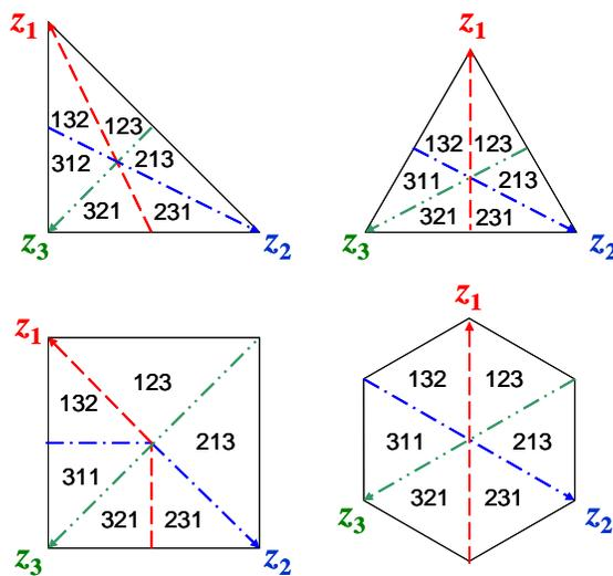
**Figure 6, center-preserving transforms.** The numbers refer to the  $q!$  piecewise continuous regions over which a transform is applicable. For example, the 132 region indicates the mixture region where  $z_1 \geq z_3 \geq z_2$ .
