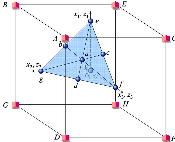
**Figure 2, correspondence of mixture and factorial space for a four-component mixture.** The four-component mixture may be mapped to the orthogonal three-factor ( $2^3$ ) factorial design space using linear transformations. Here lower case letters (spherical point markers) map to uppercase ones (cubic point markers) and vice-versa.
