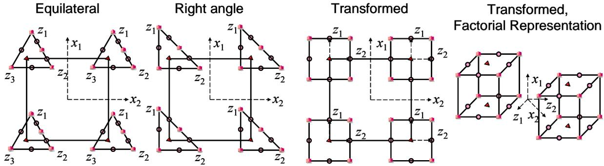
**Figure 4, illustration of a mixture-process-variable design that maps to a  $2^2 \times 3^2$  factorial design.** Point markers are segregated in three orthogonal groups. The design contains a non-uniform point distribution in the equilateral or right-angular coordinates. The mixture design is centered at  $z_1 = z_2 = 1/4, z_3 = 1/2$  rather than  $z_1 = z_2 = z_3 = 1/3$ . However, the design is symmetrical and orthogonal in the transformed coordinates.
