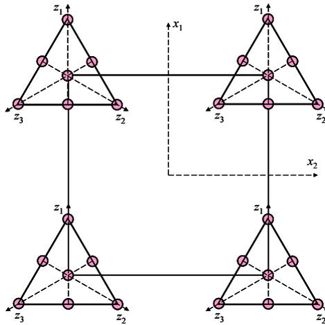
**Figure 1, an MPV experimental design.** The design represents the simplest mixture-process-variable experiment comprising interactions between two independent factors ( $x_1$  and  $x_2$ ) and three mixture components ( $z_1$ ,  $z_2$ , and  $z_3$ ).
